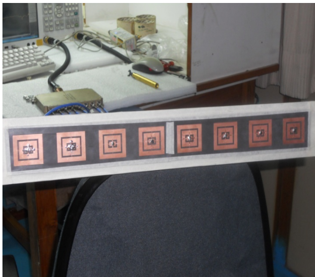
Figure 11. Photograph of Return Loss measurement Setup
