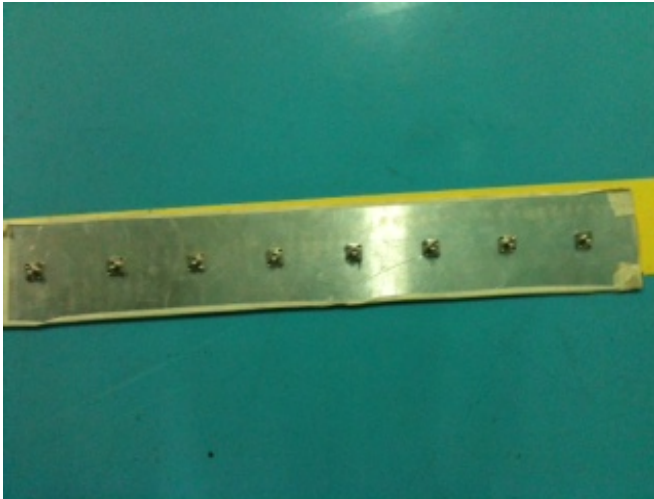
Figure 10. Photograph of Fabricated Array (Rear View)
