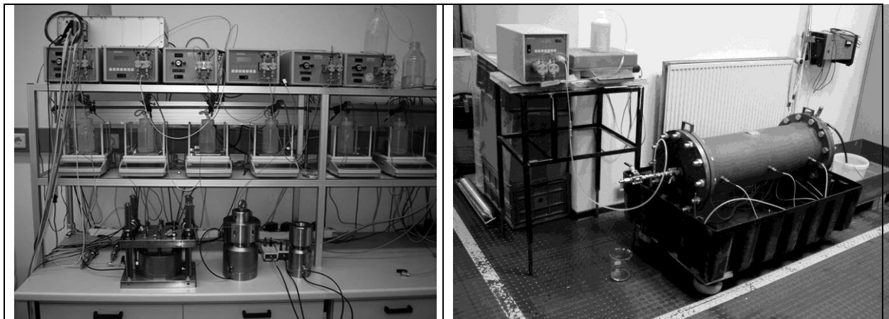
Fig. 12: Different scales of the experimental set-up for the measurement of swelling pressure of Self Sealing Backfill (SVV) in contact with brines - (left) pressure cells of different sizes and geometries, (right) large pressure tubes [10]
