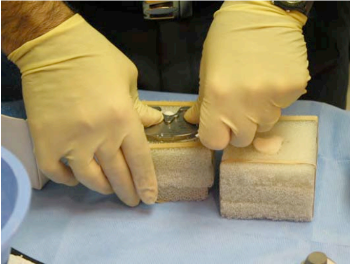
Figure 5. Preparation of the sample construct: digital pressure being applied on the cemented tibial plate. In the adjacent sample, the cement is seen filled in the reamed cavity
