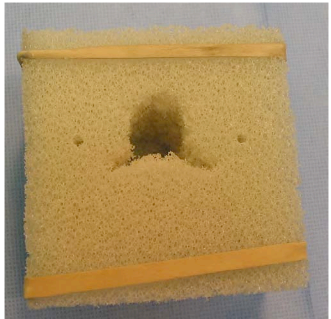
Figure 4. Preparation of the sample construct: Reamed cavity created using Zimmer prosthetic components
