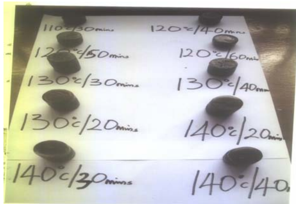
Figure-3. Polyethylene wax produced from pure water sachets showing pyrolysis temperature and time.
