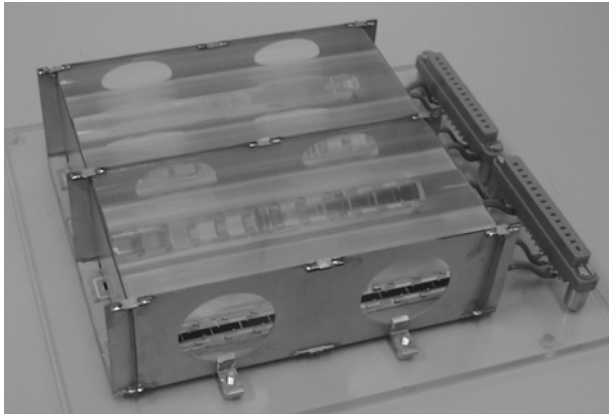
Fig. 9. Space module prototype with four linear Fresnel lenses on two glass superstrates.
