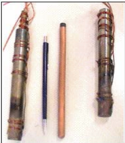
Figure 2 - Steel solid cylinder with and without a heat pipe
