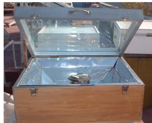
Figure 1 Solar cooker box type with internal reflectors
