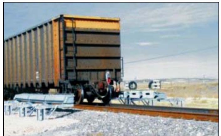
Figure 1. Trackside Acoustic Arrays
