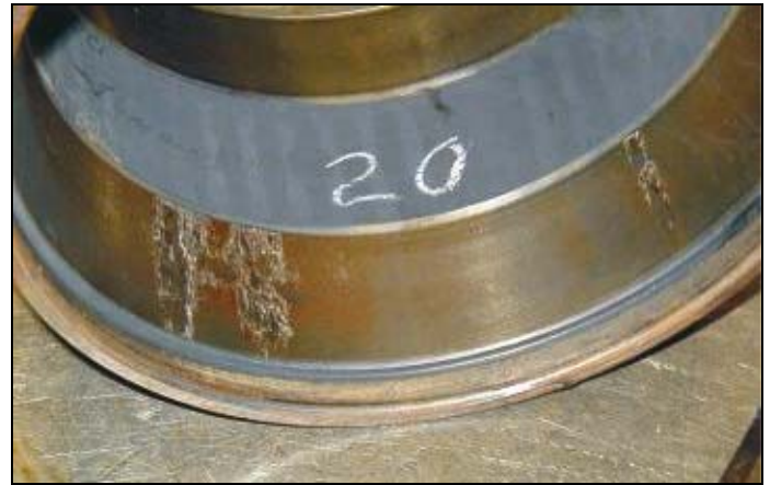
Figure 2. Raceway Spalling Example
