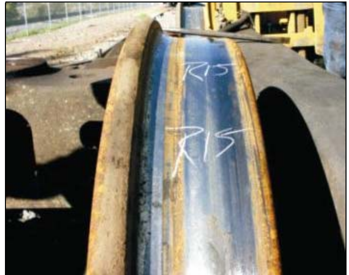
Figure 8. Wear Pattern of Wheel in Warped Truck Identified by a TPD
