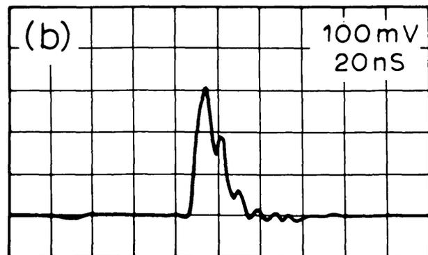
Fig. 6. (A) ArF laser pulse shape. (B) Fluorescence signal recorded at 310 nm with a photomultiplier detector.
