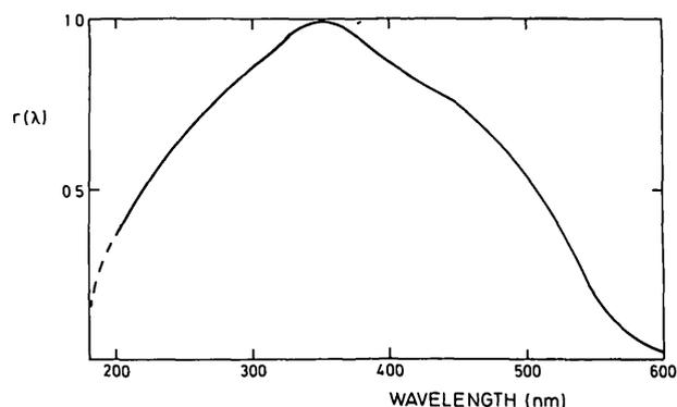
Fig. 1. Relative response ( $r(\lambda)$ ) of the monochromator detector system as a function of wavelength.
