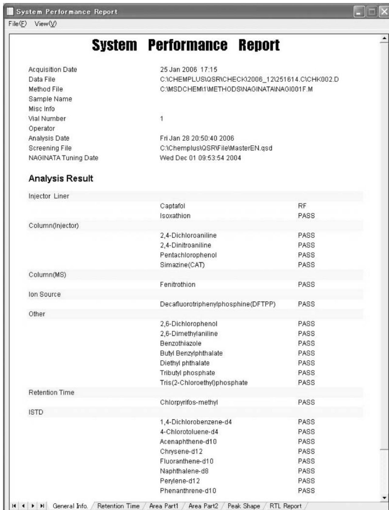
Figure 2. System Performance Report. 'PASS' indicates acceptance and 'RF' indicates rejection in each part of the instrument.
