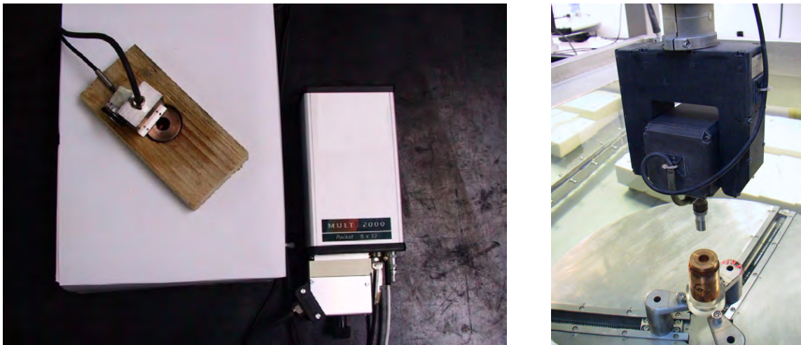
Fig. 8: 90° inspection using contact testing technique with a linear Phased Array probe (l.) and using immersion technique with a conventional probe (r.)
