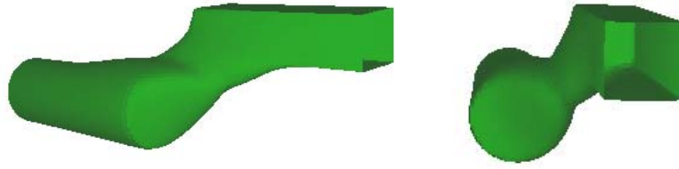
Figure 6. Bounded blending of two half-cylinders with a disk and a square as cross-sections.
