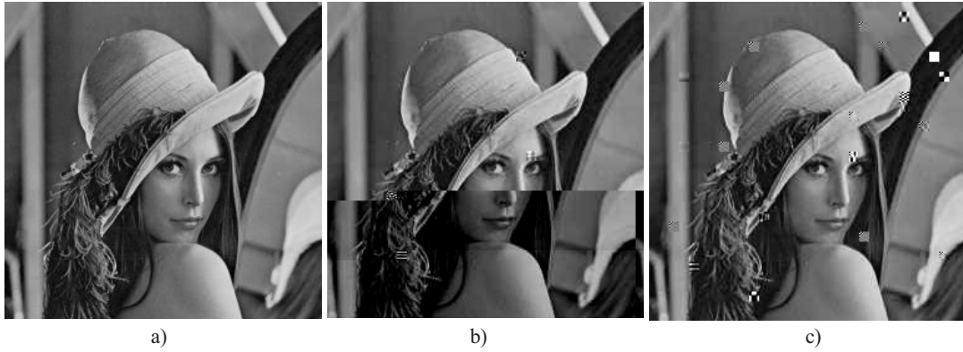
Fig. 4. Image 'Lena', when the EOB codeword is not recognized while decoding (a) original image, (b) after transmission without the restart markers, bit error rate (BER) = 0.01 %, bit rate 0.8 bpp, MSE = 1777.9 , number of bit errors = 7, (c) after transmission with the restart markers and the bit error rate (BER) = 0.05 % and bit rate 0.8 bpp, MSE = 207.7 , number of bit errors = 35.
