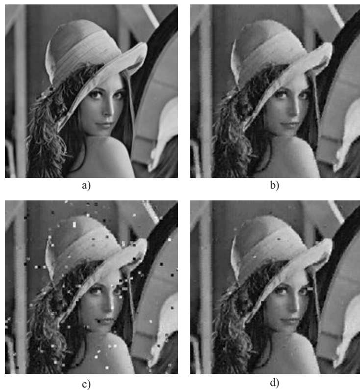
Fig. 11. Example of the SMT with sensitivity threshold = 1230 applied to the image ‘Lena’: (a) original, lossless image, (b) VQ coded image, bit rate 0.625 bit/pixel, PSNR = 26.98 dB, (c) erroneous image, BER = 0.5\% , 128 erroneous blocks, PSNR = 21.93 dB, (d) corrected image using ARQ and SMT, 74 right marked blocks as erroneous, 54 incorrect marked blocks as erroneous, PSNR = 25.18 dB, throughput = 96.85 %.
