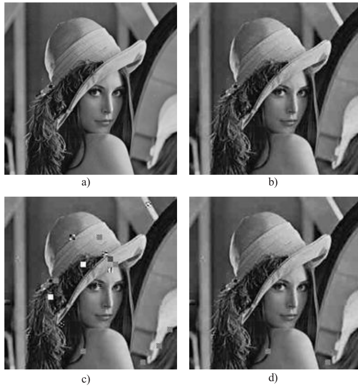
Fig. 10. Example of the SMT with sensitivity threshold = 2000 applied to the image ‘Lena’: (a) original lossless image, (b) JPEG coded image, bit rate 0.6 bpp, PSNR = 30.09 dB, (c) orrupted image, BER = 0.05\% , 22 erroneous blocks, PSNR = 23.83 dB, (d) corrected image using ARQ and SMT, 16 right marked blocks as erroneous, 4 incorrect marked blocks as erroneous, PSNR = 28.71 dB, throughput = 81.17 %.
