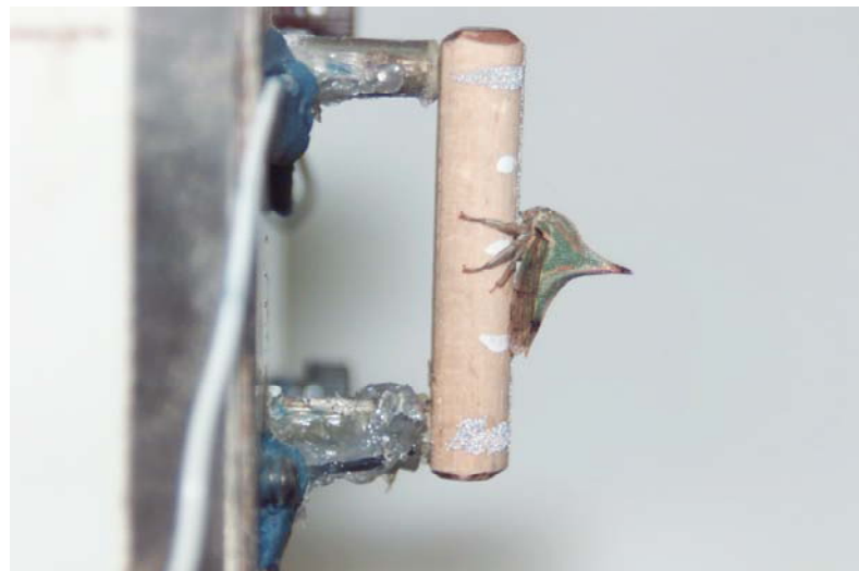
Figure 3. Stem simulator used to characterize the treehopper's mechanical response to substrate vibration.
