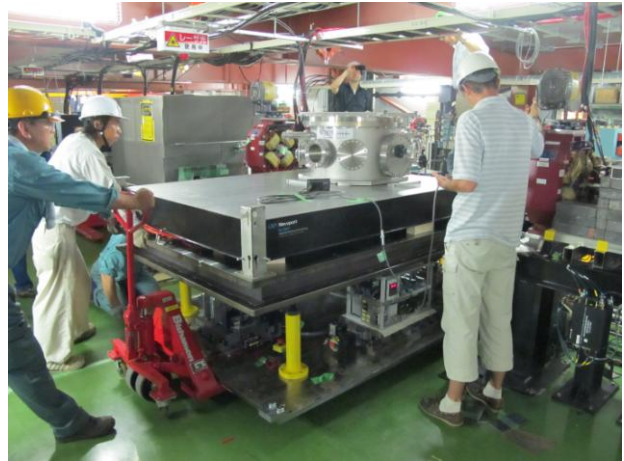
Fig 5: Installation of the four-mirror cavity in ATF.
