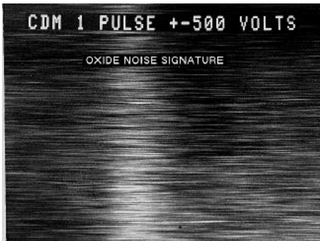
Photo 2 Typical Oxide Noise Signature associated with an input pin leakage of 220 nA at 6 Volts. Slow scan rate is 30 seconds.
