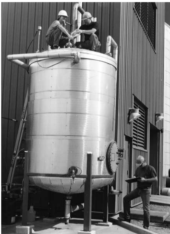
Fig. 3. An 8000-liter fermentation tank used to start the process of turning cellulosic material into ethanol. [Credit: New Energy Company of Indiana; DOE/NREL]
