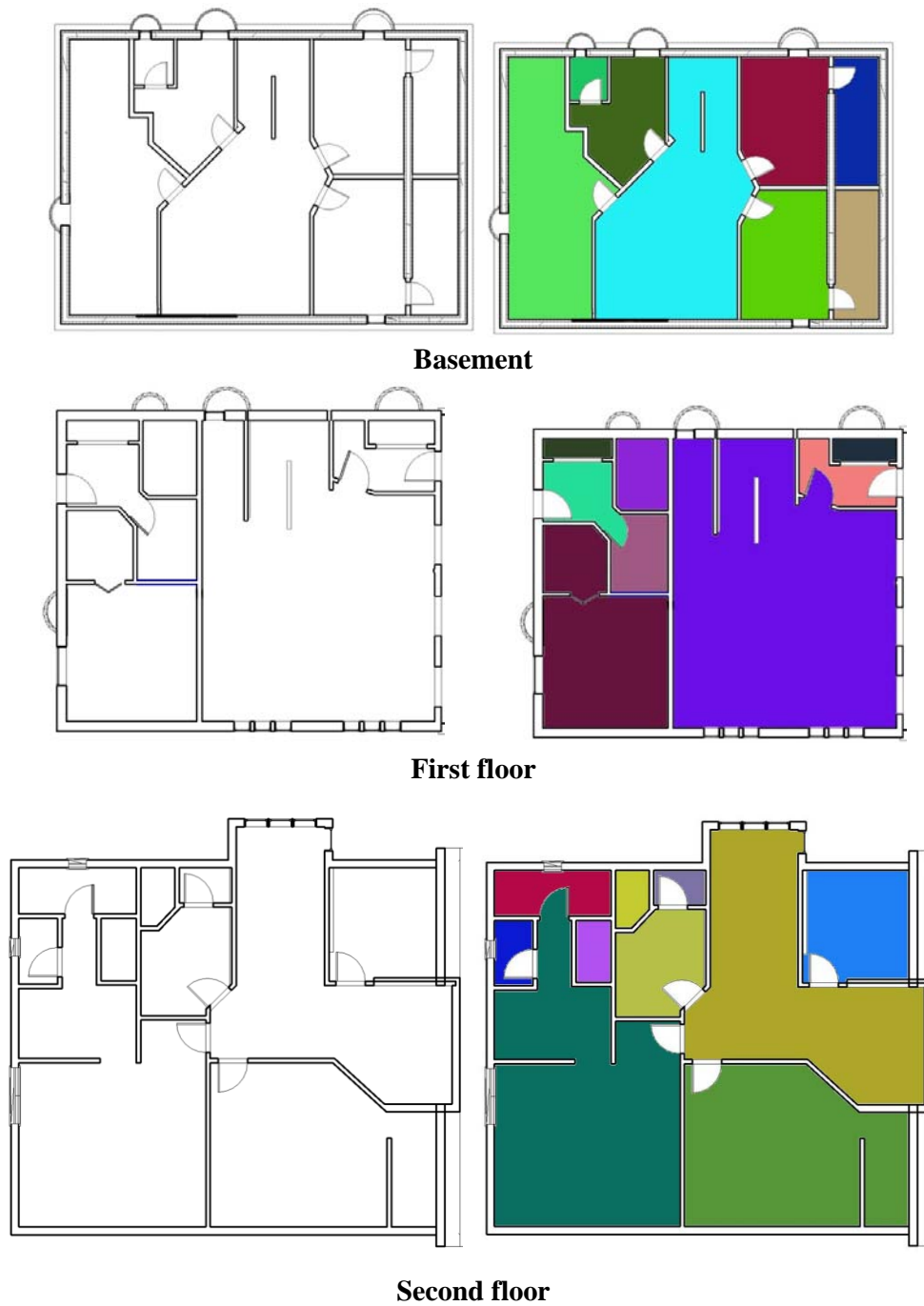
Figure 4. Original floor plan image (left) Room zone segmented floor plan image (right)
