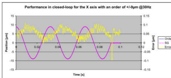
Figure 14: Comparison of order and SG response under \pm 9\mu\text{m} @30Hz.
