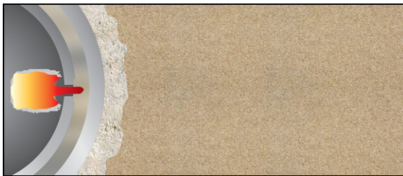
Figure 2C – Jet Penetrating Carrier Wall
