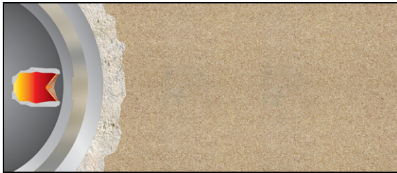
Figure 2B – Shaped Charge Detonating
