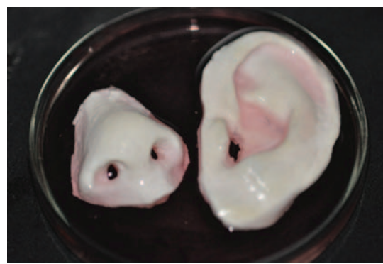
Fig. 4. Complex anatomical structures of nose and ear produced via the phase separation process with controlled porosity and mechanical rigidity using a POSS-Nanocomposite polymer developed and patented by authors.
