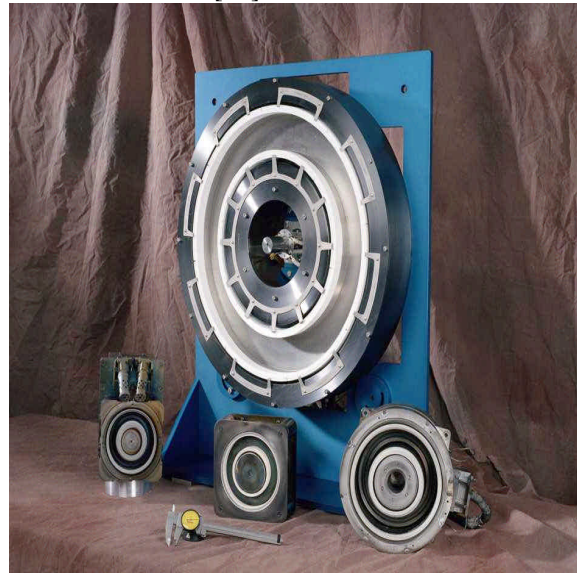
Figure 3 - NASA-457M (large thruster in the center), NASA-120M (small thruster in center), SPT-100 (left), T-160 (right).
