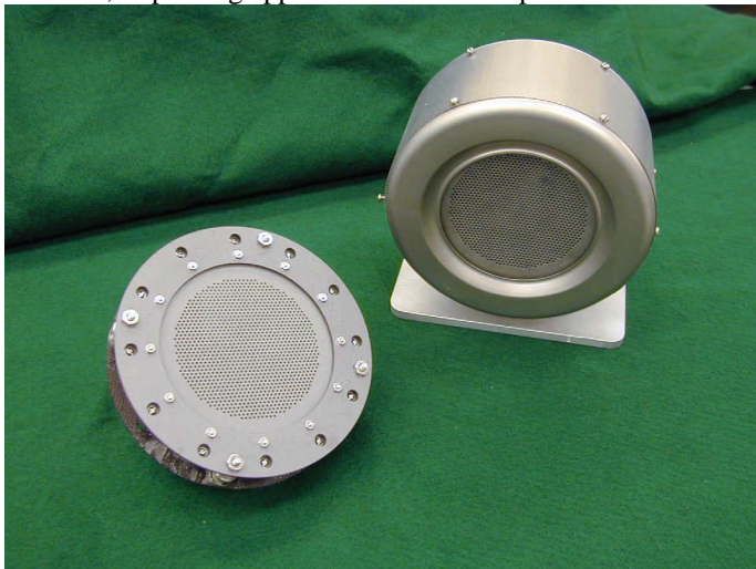
Figure 2 - 8-cm Diameter Pyrolytic Graphite Ion Optics (shown with 8-cm engine).
