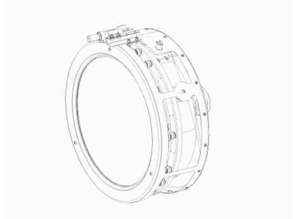
Figure 1 - Isometric Drawing of the NEXT 40-cm EM Ion Engine.
