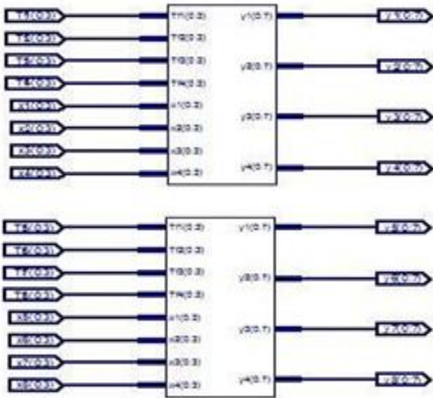
Fig.8. Even and odd parts in top radix-4.
