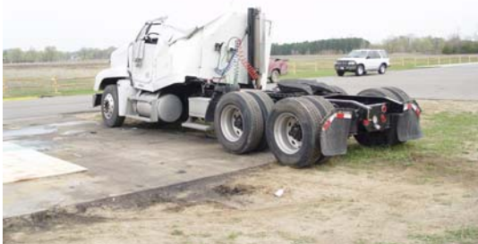
Figure 6: Exemplar roll-caged vehicle, post drop test.
