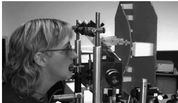
Figure 1. Schematic drawing, data, and photo of the open field wave front sensor. The subject views the fixation targets through a large hot mirror and the rest of the sensor is located below and to the side of the subject to avoid obstructing the field of view. The inset shows the setup from above during an off-axis measurement with spectacles.
