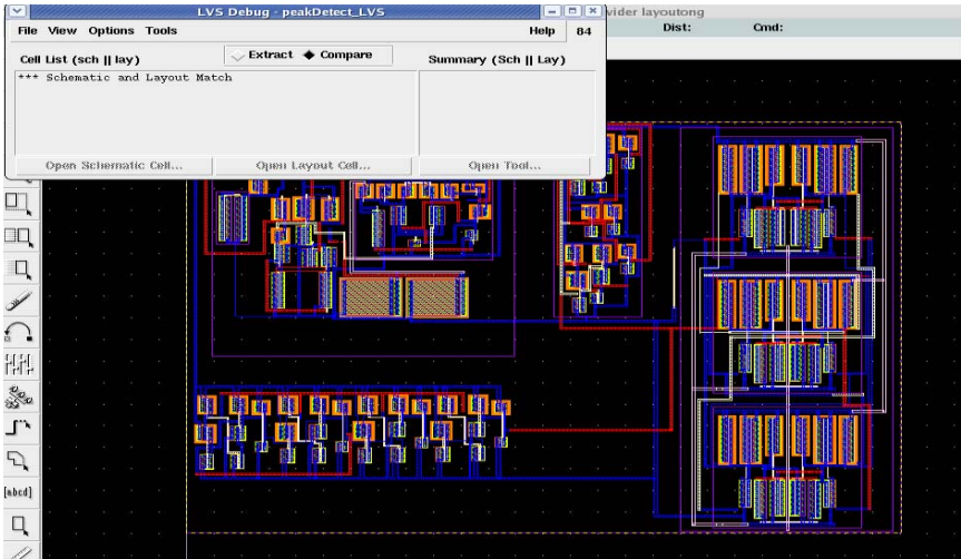
Fig. 12: Layout of complete PLL
