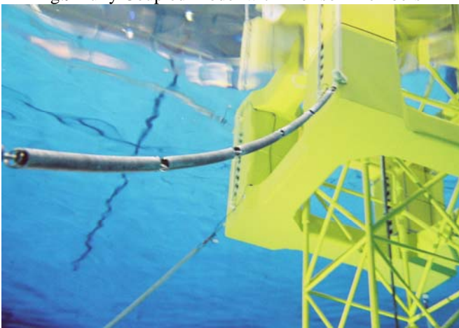
Fig.10 Under-water View of Lumped and Truncated Mooring Line
