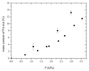
Fig. 5. The sorption isotherm of water in PA-6,6 at 300 K. The symbols represent calculations ( $\bullet$ ) and experimental data at 298 K ( $\blacksquare$ ) (Lim et al., 1999) and 300 K ( $\bullet$ ) (Watt, 1980). Figure is taken from (Eslami & Mehdipour, 2011).
