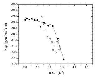
Fig. 10. Comparison of the calculated ( $\bullet$ ) and experimental permeability coefficients of water in poly(ethylene terephthalate). The experimental data are from ( $\Box$  Launay et al., 1999); ( $\bigcirc$  Shigetomi et al., 2000); ( $\diamond$  Changjing & Junying, 1987); ( $\triangle$  Rueda & Varkalis, 1995); and ( $\nabla$  Kloppers et al., 1993). Figure is taken from Eslami & Müller-Plathe (2009).
