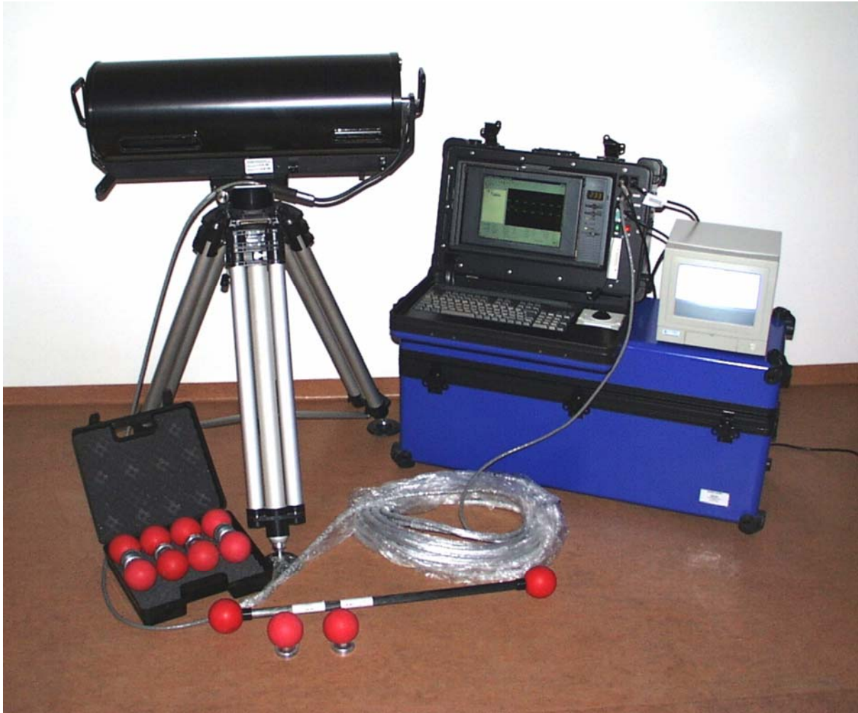
Fig. 1. A-1 Decommissioning project, Slovakia: 3-D laser scanner
