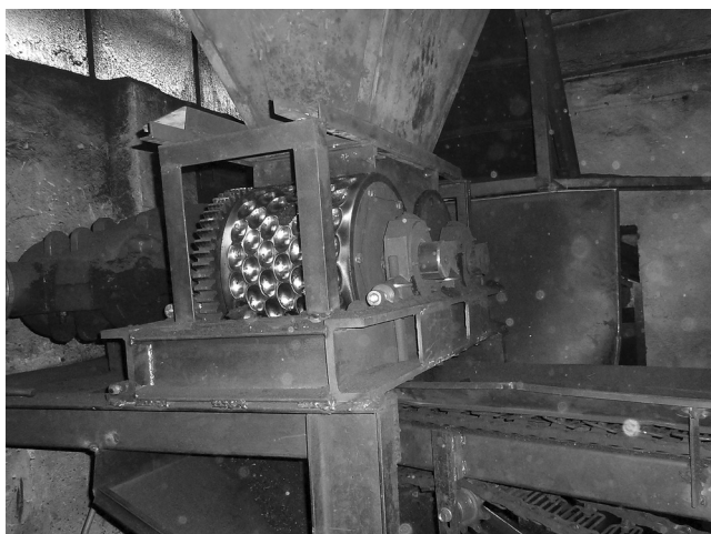
Figure 1. Work rolls system in the briquetting press.
