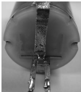
Figure 12. X2Y ® component prototyped on the outside of the washer-pump. (Note: the prototyped motor used a 1014 size X2Y ® for easier attachment).
