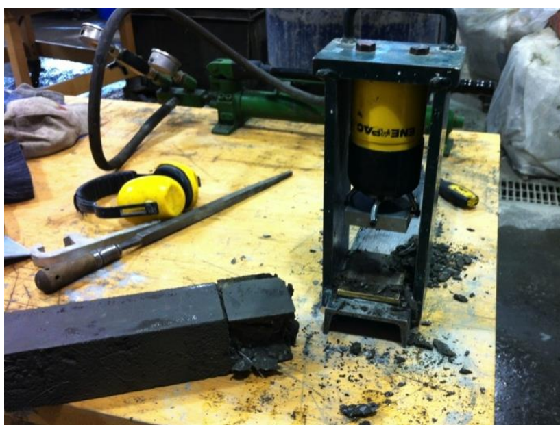
Figure 4 End beam test apparatus
