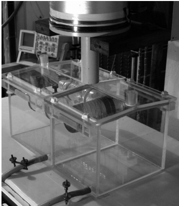
Fig. 1. Configuration of the phantom of thorax and abdomen consists of two containers filled with distilled water, models of lungs and liver. A part of the SQUID system is shown above.
