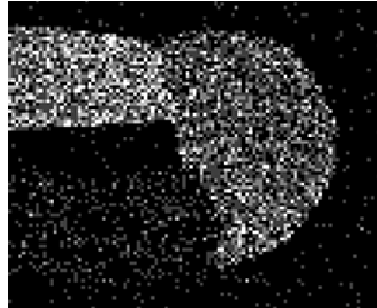
Figure 2. Elemental mapping from SEM-EDX analysis of chromium content in a type K thermocouple
