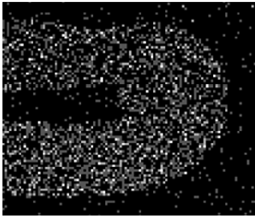
Figure 4. Elemental mapping from SEM-EDX analysis of manganese content in a type K thermocouple
