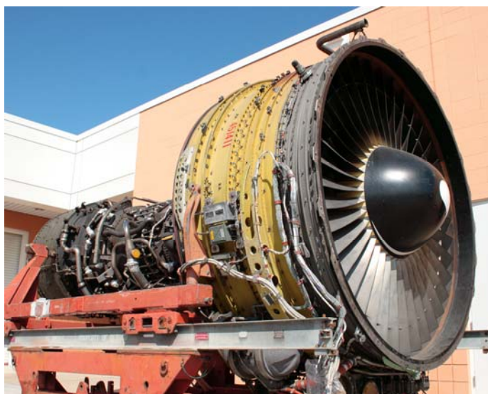
Figure 1. General Electric CF6-6 high-bypass turbofan engine located at the Gas Turbine Laboratory at the Aerospace Engineering Dept of Embry-Riddle University.
