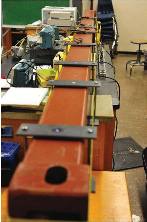
Fig. 4. Corner post setup showing two corner posts held in compression with hand hoist and (yellow) nylon strapping. Shown in the picture are seven transducers mounted along the length of the corner posts.
