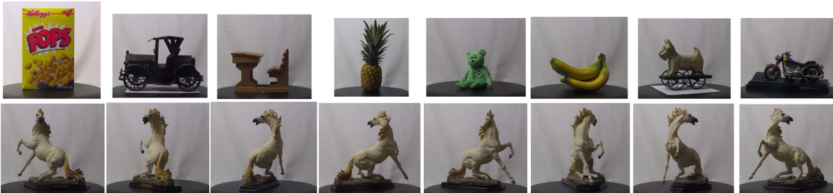
Figure 8: Our calibrated database consists of photographs of 100 objects which were imaged in three lighting conditions: diffuse lighting, light from left and light from right. We chose our objects to represent a wide variety of shapes and surface properties. (Top) Eight sample objects from our collection. (Bottom) Each object was rotated with 5^\circ increments and photographed at each orientation with both cameras and three lighting conditions for a total of 72 \times 2 \times 3 = 432 photographs per object. Eight such photographs are shown for one of our objects.
