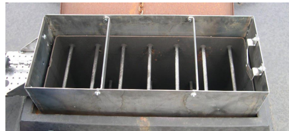
Figure 2. Exhaust Stack Extension
