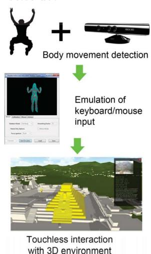
Figure 3. The system set-up, with the Kinect device recording the human movements and FAAST emulatating the keyboard input to control the QueryArch3D tool.
