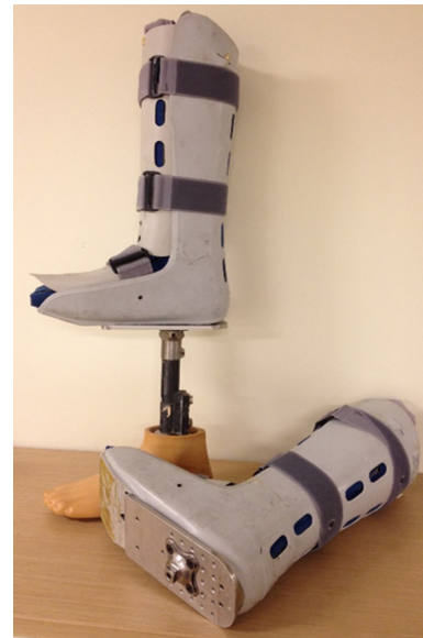
Fig. 2 Walking simulator boots. Prosthetic components attach distal to the foot plate and mimic transtibial prosthesis use.
