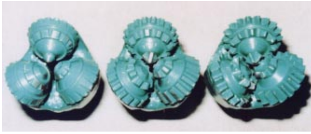
Fig. 1 Milled-tooth bits of 98.43-mm (3-7/8-in) diameter (from left: T7, T4, T0)
