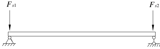
Figure 6. schematic drawing when support forces are independent
