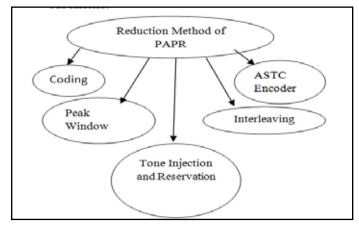
Fig. 1: Method of Reduction PAPR
