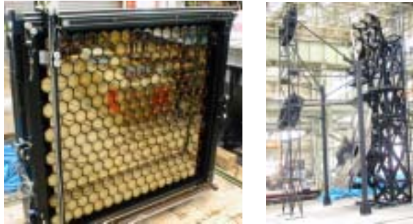
Fig. 1. The prototype camera and telescope reflector for the fluorescence measurement.
