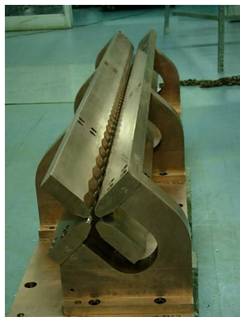
Fig. 1 Fabricated Model of Prototype RFQ
