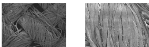
Figure 5a: SEM image of invitro biodegradation- PHB with gelatin textile laminate
