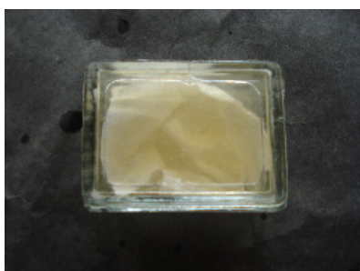
Figure 2a: Coating of PHB with gelatin starch on textile fabric
