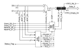
Figure 6. Architecture of Input part of Router.
