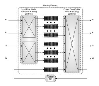
Figure 2. System Level specification of Router Architecture.
