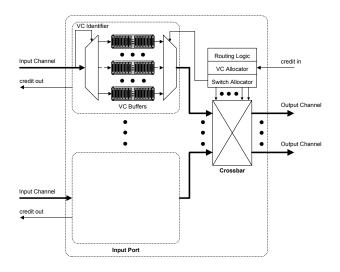
Figure 1. Typical Virtual Channel Router Architecture.
