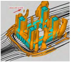
Figure 7 - Typical vortex flow around a platform
