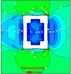
Figure 8 - Velocity amplifications around a platform
