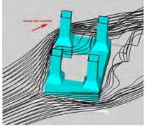
Figure 6 - Typical streamlines around a platform
