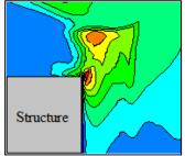
Figure 5 – Example of shear stress amplifications
