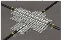
Figure 3 – Mattress underneath a pipeline
