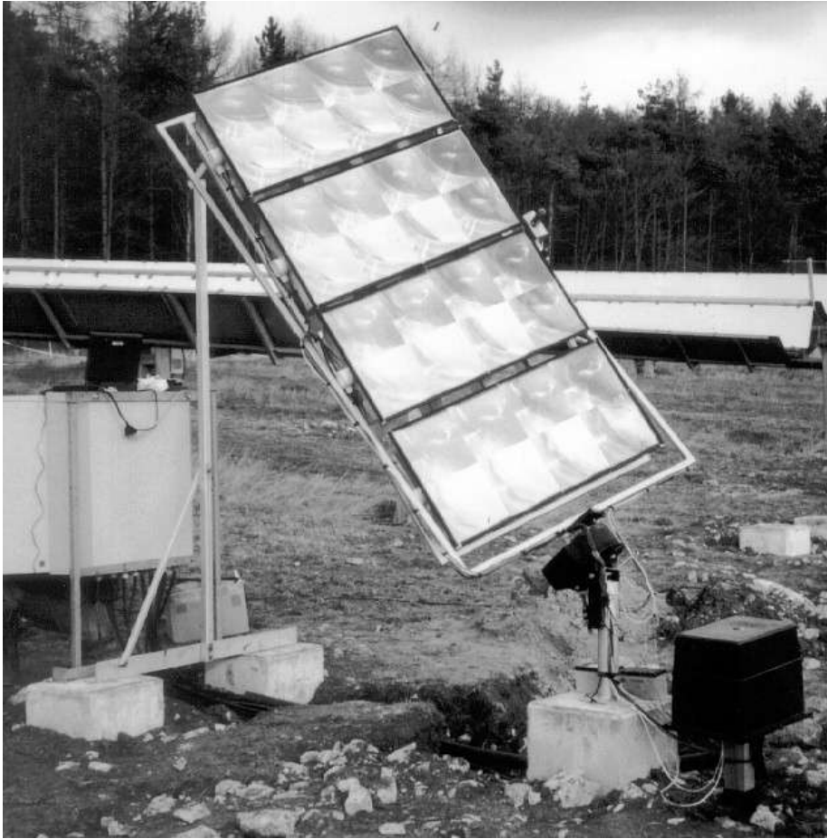
Figure 3. Collector A. Multiple point focus Fresnel lenses, mounted in gimbals, with closed-loop tracking about both axes.
