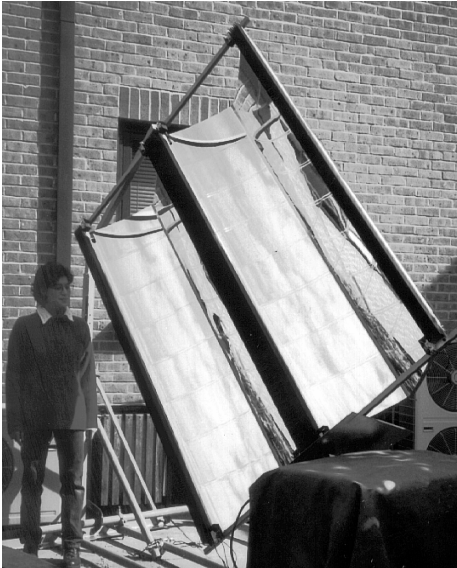
Figure 7. Collector C. The single-mirror two-stage collector, tracking about a polar axis.
