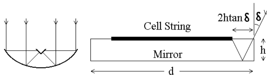
Figure 1. Shading loss: the cell string has to be shorter than the collector.
