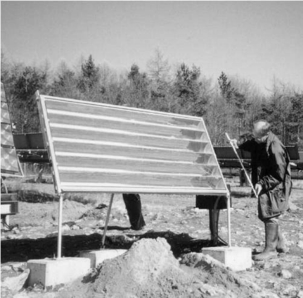
Figure 9. Collector F. Multiple cylindrical semi-parabolic mirrors, moved manually every day about an E-W axis.
