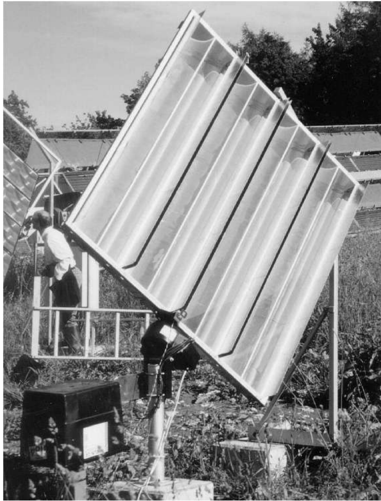
Figure 5. Collector B. Multiple cylindrical semi-parabolic mirrors, tracking about a polar axis.
