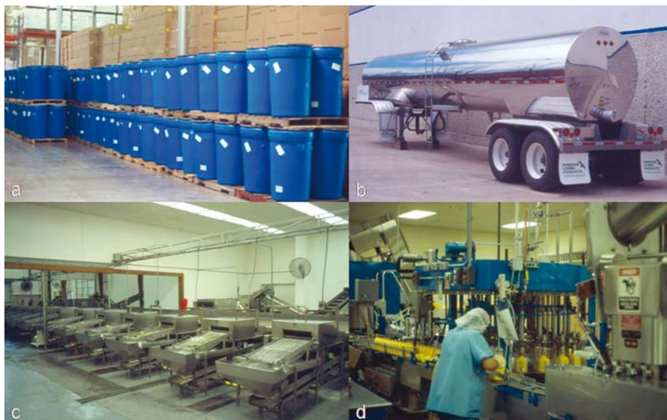
Figure 2. Large-scale production of Aloe vera gel. a, bulk aloe gel for export; b, refrigerated bulk trailer for transporting fresh gel to the factory; c, mechanical filleting of aloe leaves; d, bottling of the gel as a health drink.
